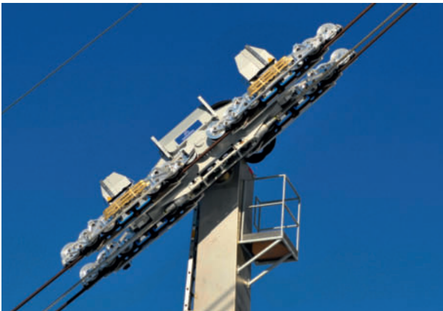
The new lightweight 24-wheel carriage from Garaventa for the Säntis aerial tram
