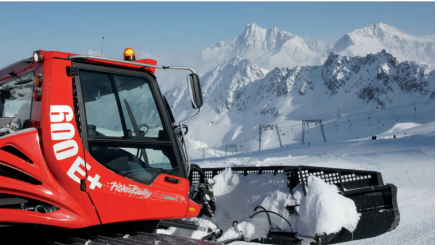
PistenBully 600 E+ – the first groomer with a diesel-electric drive at work on the mountain
