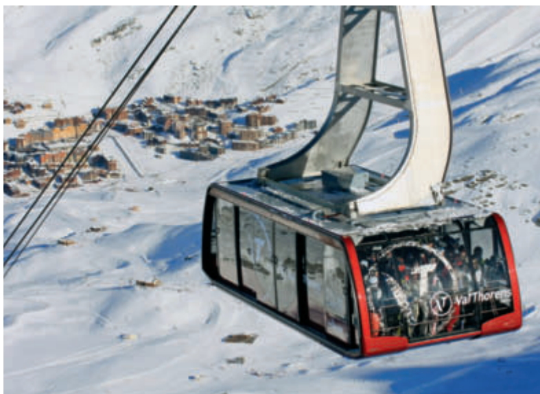
At the end of 2012 two Gangloff cabins were delivered to the Val Thorens – Cime de Caron jigback. The convex shape of the all-round laminated glass windows gives the cabins a dynamic touch.
