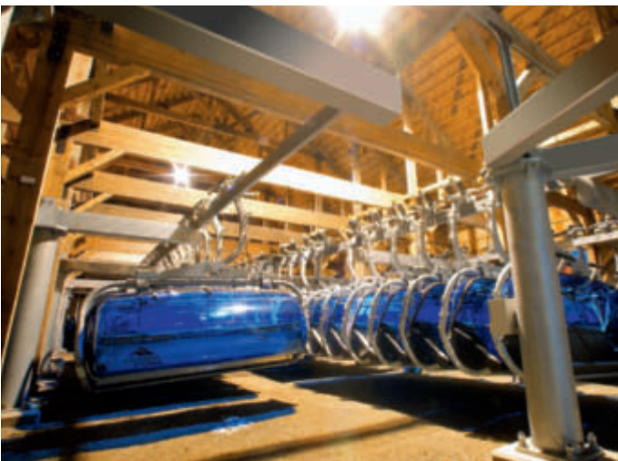
Parking barn parking neatly stores bubble chairs for protection and opening efficiency.
